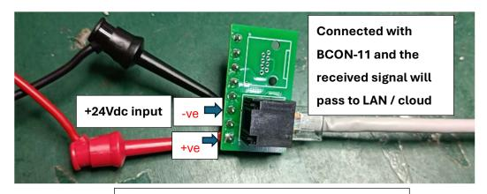
Power input and cable connection to BCON-11
