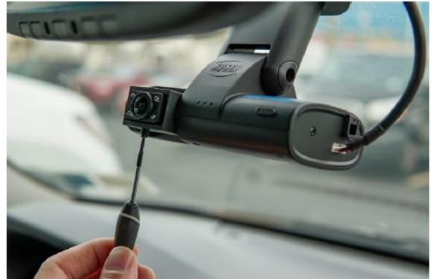
6 - Using a T-15 security bit, loosen the set screw on the bottom of the camera to adjust your view
