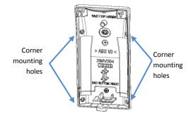
Use only 2x screws on the same side (left or right) to mount the casing on the corner
