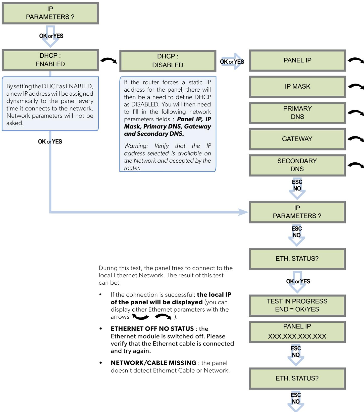
During this test, the panel tries to connect to the local Ethernet Network. The result of this test can be:
