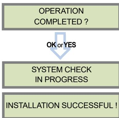
Before completing programming make sure that no device is tampered. Each device must be closed and its LED indicator shall be turned off.
