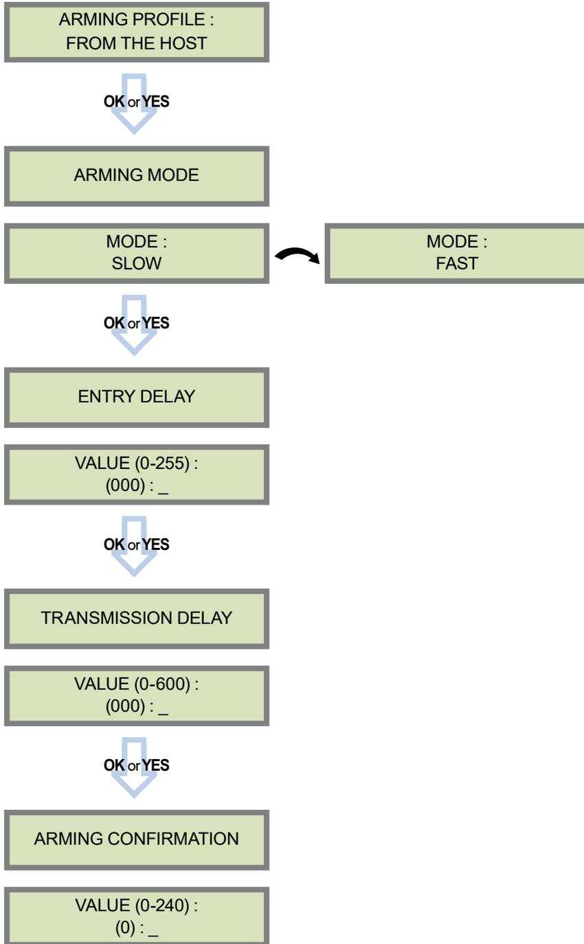
**MODE SLOW** : The panel will arm each device one at a time saving battery life. We recommend this mode.
