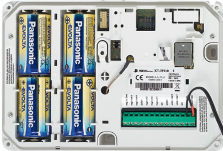
In this functioning mode, the XTO-iP panel works as a standard hybrid alarm system with 25 wireless peripherals and 3 programmable inputs. It is a totally standalone alarm system.
