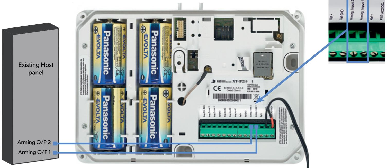
When the panel is used in XTENDER mode, the system will only be able to arm and disarm by latching 9-12Vcc to its arming inputs Arming Input 1 and/or Arming Input 2.
