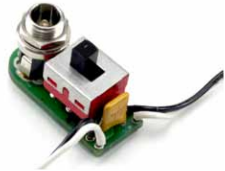
Battery Switch / Charging Module
