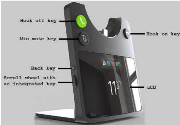
Fig.3 RTX745x front view
