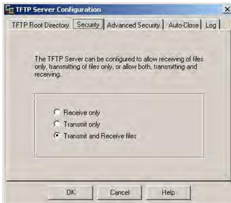
**NOTE:** If TFTP server timeout settings are too short firmware upgrade might not complete. Recommended time out setting is more than 3 seconds.
