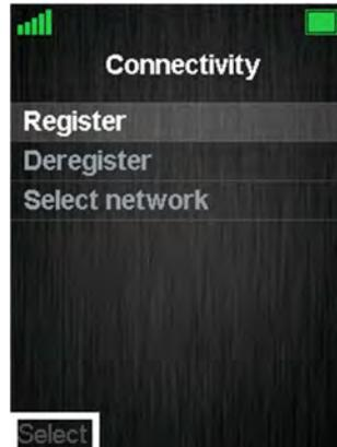
c) Select an empty spot in order to register the handset and enter the “Access code” which by default is “0000”.
