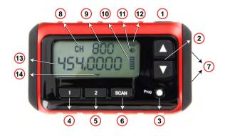
Power On/Off Button Volume or Channel Up/Down Buttons 2 3 Programming Button 4 Channel 1 Preset <u>Button</u> 5 Channel 2 Preset Button 6 Scanning modes Button 7 IN (Auxiliary Audio Input), OUT (Earphone Jack) 8 Channel or Sub Channel Indicator Ohannel Number Display 🔟 Volume Level Bars 11 **Communication Indicator** 12 Low Battery Indicator 13 Frequency Display Preset or Scan Mode Selection Indicator 14
