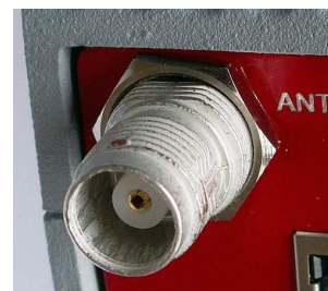
Fig. 4.4: Antenna connector TNC
