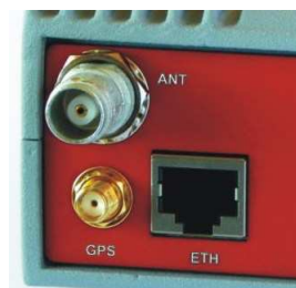
Fig. 4.12: GPS Connector SMA
