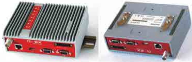
Fig. 6.1: Flat lengthwise mounting to DIN rail – recommended
