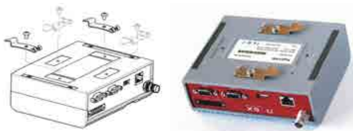
Fig. 6.2: Flat widthwise mounting to DIN rail
