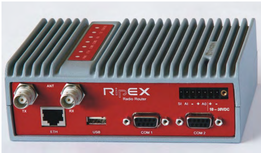
Fig. 4.7: Separated Rx and TX antennas
