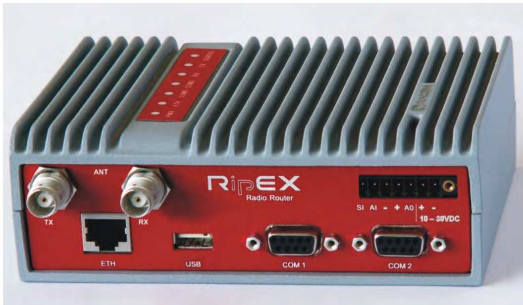
Fig. 4.7: Separated Rx and TX antennas
