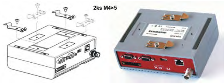
Fig. 6.2: Flat widthwise mounting to DIN rail
