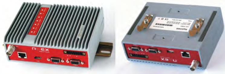
Fig. 6.1: Flat lengthwise mounting to DIN rail – recommended
