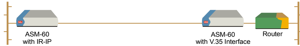
Figure C-1. Typical Application of ASM-60 with IR-IP
