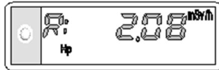
Figure 9 Display of Dose Rate in Measurement Mode
