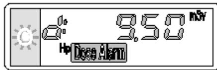
Figure 5 DMC 2000TD LCD Display Indication
