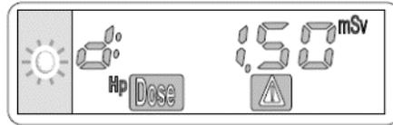
Figure 32 Simulated Dose Pre-Alarm Display
