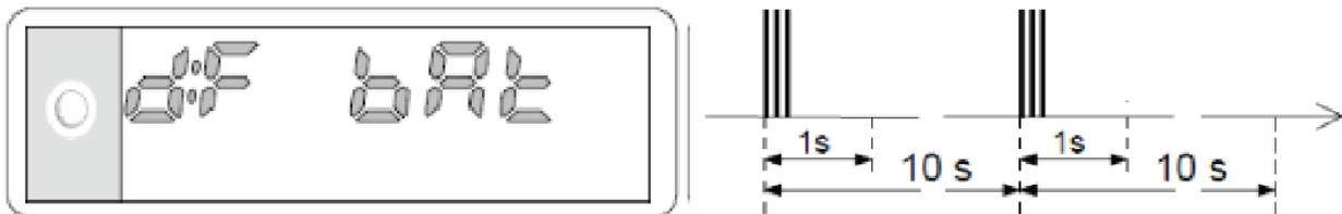
Figure 47 Simulated Defective Battery Fault Display and Sound
