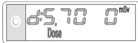
Figure 23 DMC 2000TD Simulated Cumulative Dose Display
