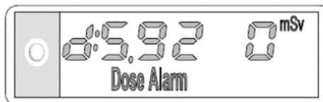
Figure 25 DMC 2000TD Simulated Dose Alarm Threshold Display
