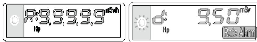
Figure 11 Dose Equivalent Rate Saturation Display
