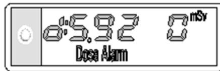
Figure 13 Simulated "Dose" Alarm Threshold Display
