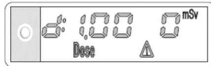
Figure 27 DMC 2000TD Simulated Dose Pre-Alarm Threshold Display
