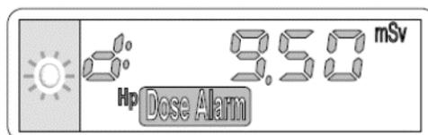
Figure 35 Simulated Dose Alarm Display
