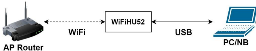
Figure 46 Test WiFi environment under Ubuntu 16.04 Linux
