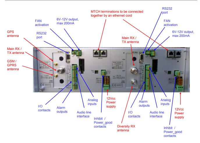
For this example, the following picture shows how two repeaters should be connected to implement a simulcast network with <u>UHF links</u>. Two ethernet patch cord are needed to connect together the MTCH ports and the ethernet ports of the two radios; they are represented in pink color.
