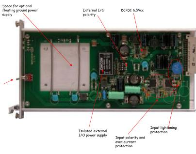
Equipment is power supplied by nominal 13,8Vdc from battery with negative shorted to ground and with a maximum current absorption of 5 A. In case of other power supply sources, other PSU models are available, DC/DC (nominal 12-24-48V, isolated) or AC/DC (nominal 220V) with battery charger.
