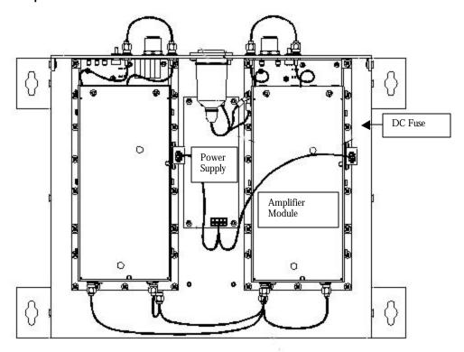
Only the power supply is field replaceable part number 31500012900
