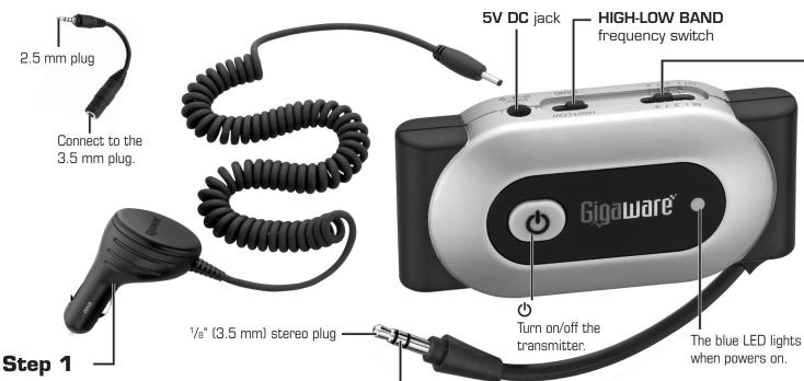
Connect the 12VDC plug into your car's power port. Conect the other end to the **5V DC** jack on the transmitter.
