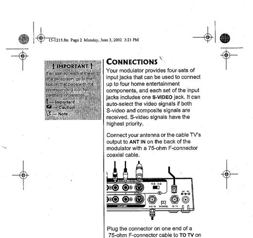
the back of the modulator, and plug the connector on the cable's other end to
