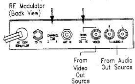
Turn on the input source (such as video camera or VCR etc.) and set OHMS 75/1k on the RF Modulator to the position that gives the best picture.
