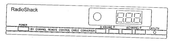
Press POWER to turn the converter and the switched AC outlet on and off. When the converter been turn off, a LED dot (at lower right corner) is lit up to indicate the converter is in standby mode.
