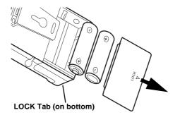
1. Move the **LOCK** tab in the opposite direction of the marked arrow on the bottom of the transceiver.
