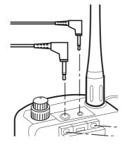
**Note:** Inserting the headset plug automatically disconnects the internal speaker and the push-to-talk (PTT) button.
