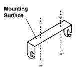
Note: If you cannot reach behind the mounting surface to attach the nuts on the bolts, use the 1/5-inch (5-mm) tapered-tip screws and plain washers to secure the bracket.
