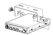
Note: The radio has a Compass mode and in order to use the mode correctly, You have to install this set HORIZONTALY.
