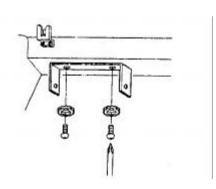
4. Attach the CB to the mounting bracket using the supplied rubber washers and mounting knobs.
