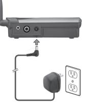
If you use rechargeable batteries, the intercom will automatically recharge them whenever the AC adapter is plugged in and the **RECHARGE** switch is set to
