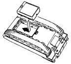
③ Install the Ni-Cd cassette pack in the battery compartment as shown in the diagram. The Ni-Cd cassette pack is designed so that the + and – poles must be positioned properly or else the pack cannot be installed.
