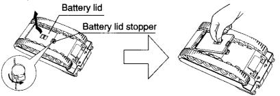
1 Turn the battery lid stopper with a coin, as shown in the diagram.
