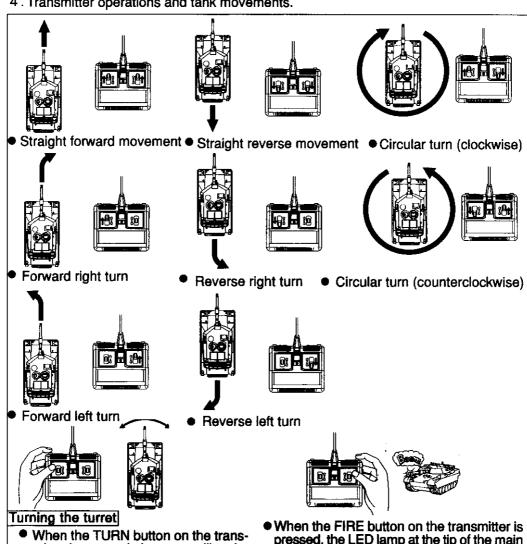
mitter is pressed, the turret will make repeated turns to the left and right.
