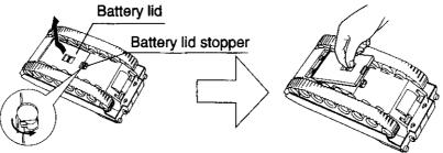
① Turn the battery lid stopper with a coin, as ② Pull up the battery lid to open. shown in the diagram.
