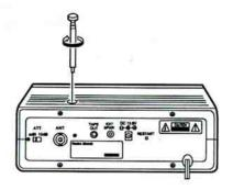
The scanner's sensitivity depends on the antenna's length and various environmental conditions. For the best reception of the transmissions you want to hear, adjust the antenna's length.
