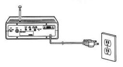
Caution: To prevent electric shock, the plug's blades are polarized and fit only one way. If the plug does not fit easily, turn it over and try again. Do not force the plug into the AC outlet.
