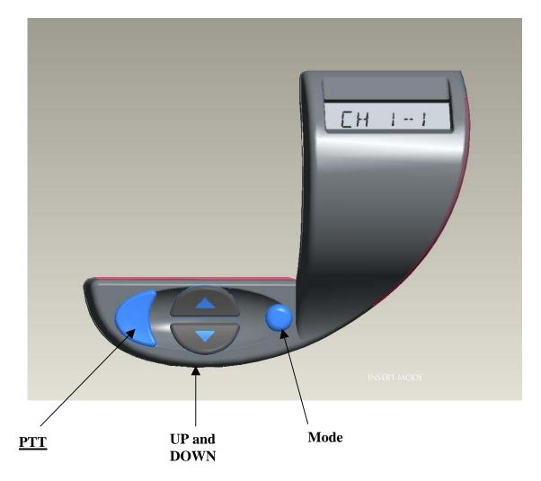
**PTT:** Pushing the Press to talk (PTT) button places the transceiver in transmit mode.
