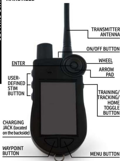
**HANDHELD:** Receives and displays location updates from the GPS Module. It sends the radio signal to the E-Collar module. It is waterproof and can be submerged in water to a depth of 5 feet.
