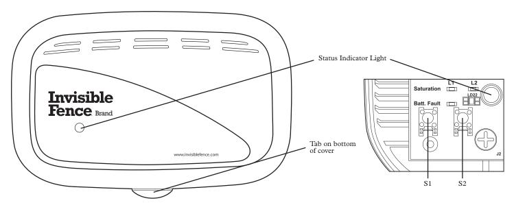
**Audible Alarm:** There is an audible alarm for certain alert conditions (see chart below). Pressing either the S1 or S2 button on the transmitter circuit board will silence the alarm. The alarm will re-activate on power-up if a failure condition still exists. Access S1 or S2 by gently pulling the tab at the bottom of the cover towards you. Once released at the bottom, the top will come off the base.
