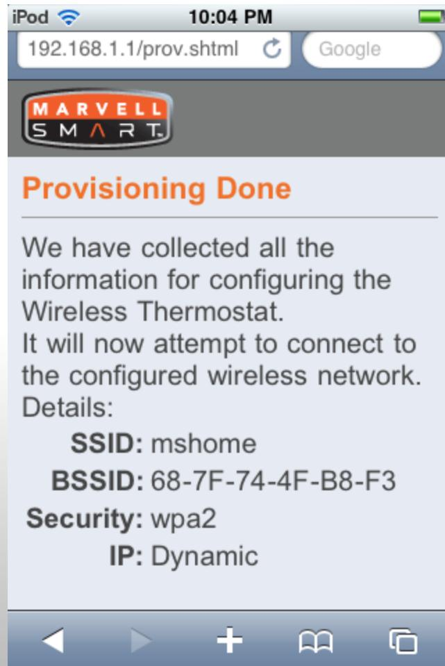
Check your thermostat. After a little bit it will blink Green. And, you will see Link under the radio tower icon. That means the thermostat is now connected to your home network.
