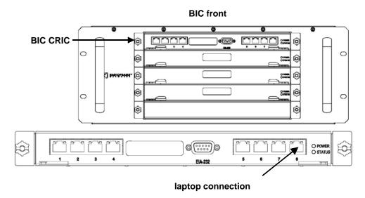
1 Connect the laptop to port 8 of the BIC CRIC using an Ethernet (CAT5) cable.
