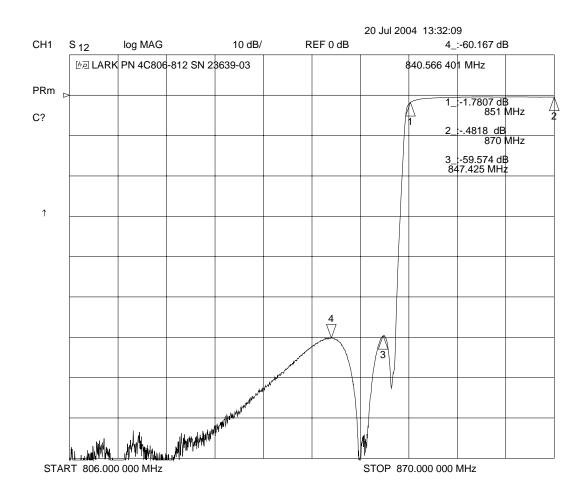
Figure 28 Transmit filter frequency response
