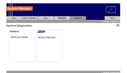
**3** On the Bit Error Rate Test page, select the RadioBlade that is to be tested.
