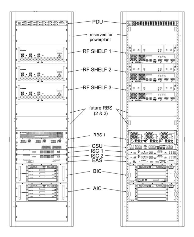
Figure 25 MC-Series System rack locations for non-RFN hardware
