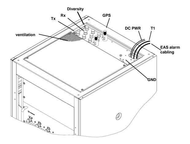
Figure 26 Top of the rack (TOR) cabling and equipment
