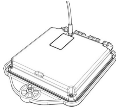
Figure 4.13 Charging the transmitter Li-Ion battery pack
