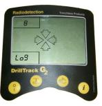
To add a simulated locate point, in the "Two Arrow Steering" screen press the key, the display will show ADD and LOG with a rod number, press key again to confirm the addition of the simulated locate point.
