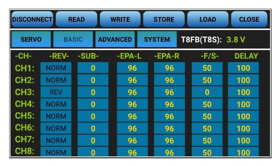
**REV:** Defines the relationship between the transmitter controls and the receiver output for channels with options of NORM and REV. Make sure to check all servos move to the correct direction as wish under control. Make sure to check all servos move to the correct direction under control.
