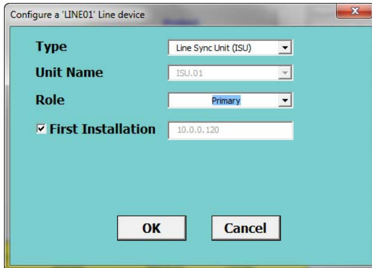
Figure 4-19: ISU - First time installation
