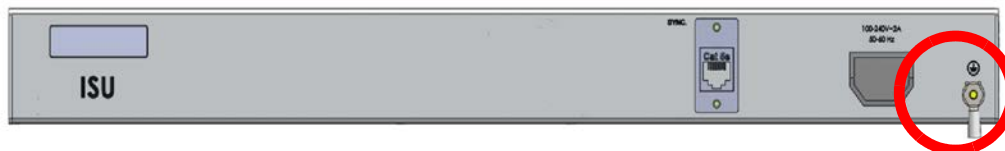
Figure 2-88: ISU: Grounding lug location
