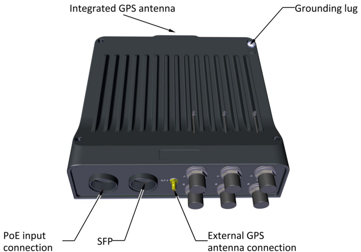
Figure 2-51: OSU external connections
