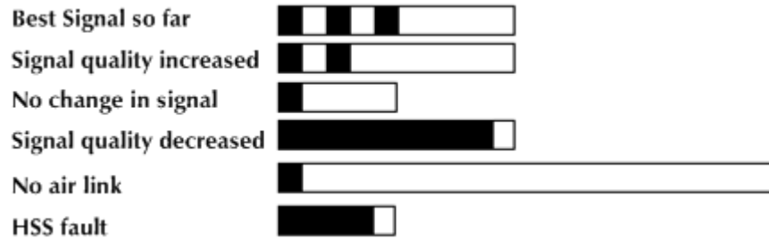
Figure 3-8: Beeper Sequence for ODU Alignment
