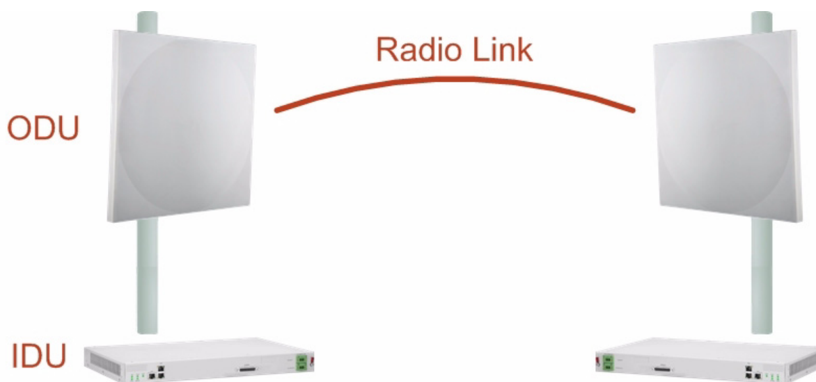
Figure 1-4: Example of Link Architecture - System Components
