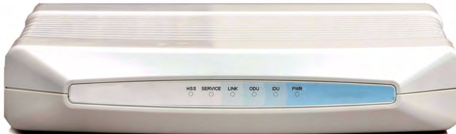
Figure 1-5: New style IDU-E - front view (Note new HSS LED on the left)
