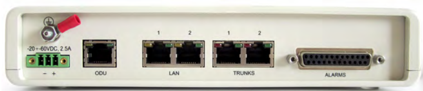
Figure 3-9: New style IDU-E: Rear panel
