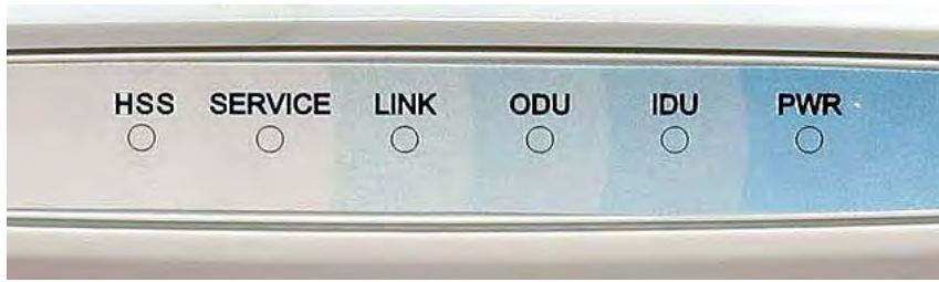
Figure 3-12: IDU-E Front Panel LEDs
