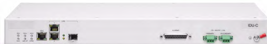
Figure 1-7: IDU-C, Ethernet only, front panel
