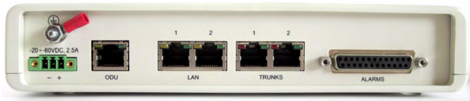
Figure 1-6: New style IDU-E: Rear panel
