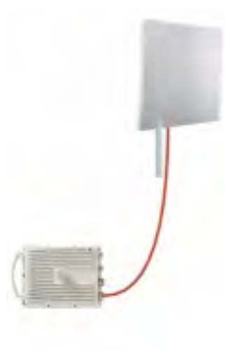
Figure 17-7: Incorrectly mounted ODU (No “water nose”)
