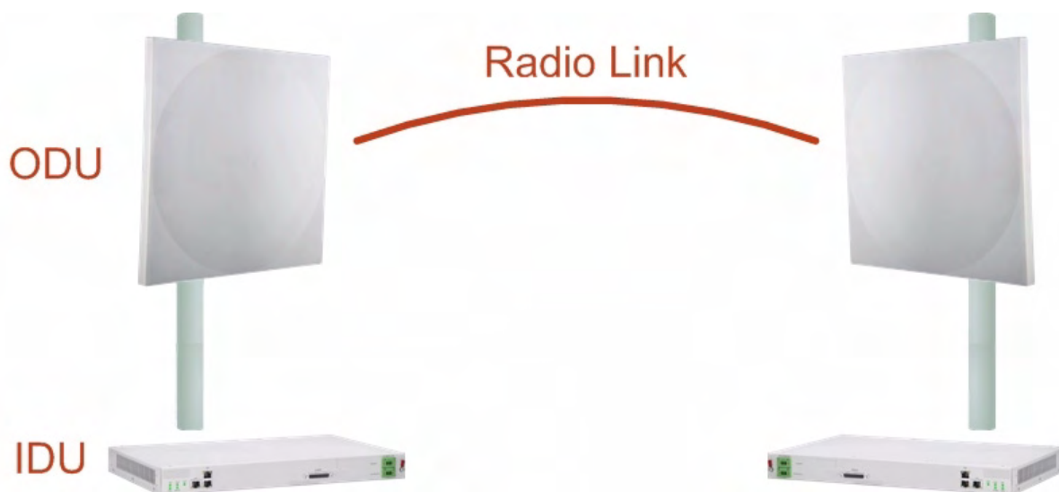
Figure 1-4: Example of Link Architecture - System Components
