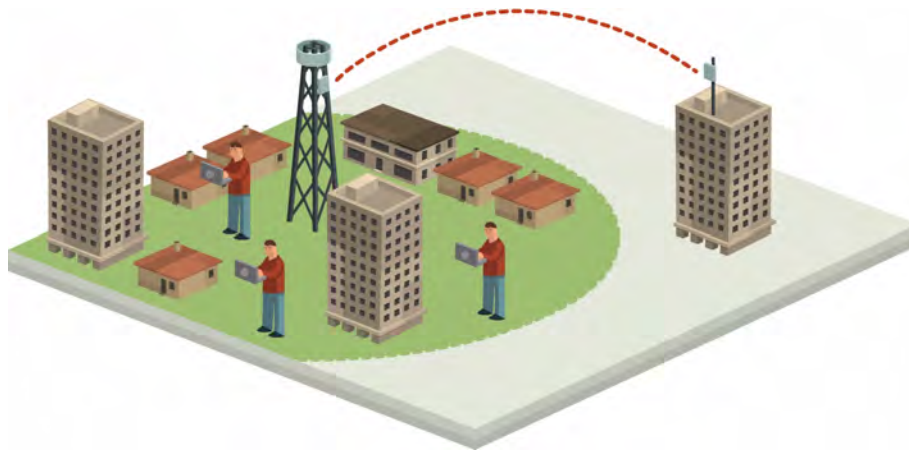
Figure 1-1: Typical Wimax and IP Backhaul application
