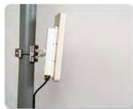
Figure 1-10: ODU with integrated Flat Panel antenna
