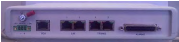
Figure 3-7: New style IDU-E: Rear panel
