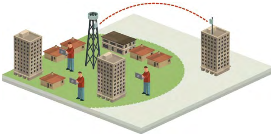
Figure 1-1: Typical Wimax and IP Backhaul application
