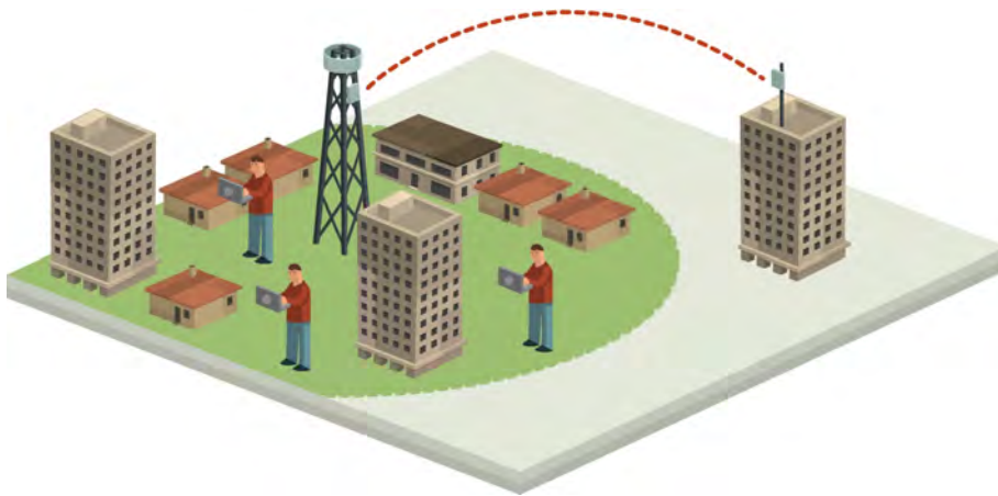
Figure 1-1: Typical Wimax and IP Backhaul application
