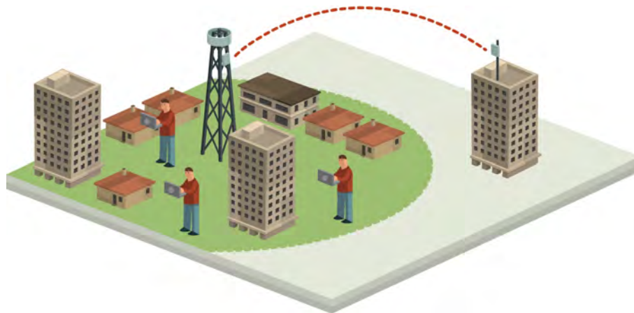
Figure 1-1: Typical Wimax and IP Backhaul application
