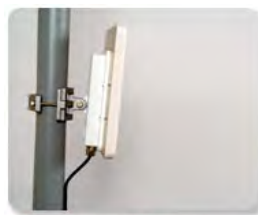
Figure 1-10: ODU with integrated Flat Panel antenna
