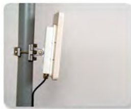
Figure 1-10: ODU with integrated Flat Panel antenna
