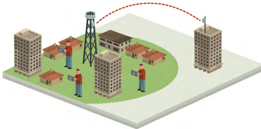
Figure 1-1: Typical Wimax and IP Backhaul application
