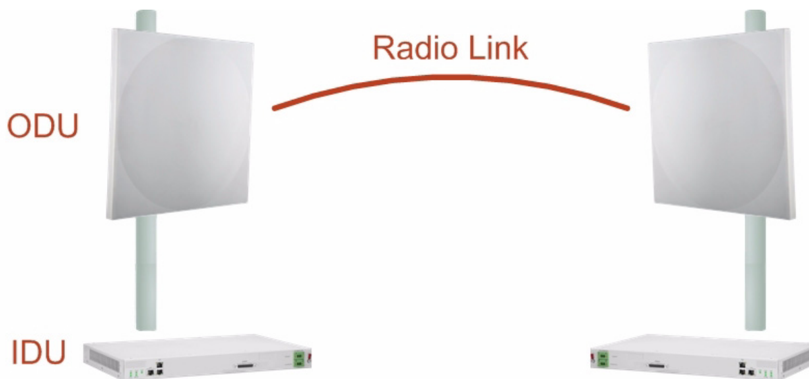
Figure 1-4: Example of Link Architecture - System Components
