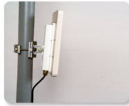
Figure 1-8: ODU with integrated Flat Panel antenna
