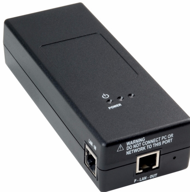
Figure 1-7: PoE device - showing the radio Ethernet port
