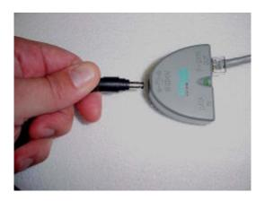
**Step 4:** Check the front panel of the indoor unit to make certain that the power LED is on. If the power LED is not on, confirm that the power cable is securely connected and that your power source is operational.
