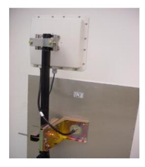
**NOTE** All external antenna configurations will come with an N-type Bulkhead adapter installed at the bottom of the main radio enclosure.
