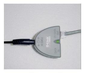
**Step 5:** Plug your Ethernet patch cable into the Ethernet input port (**Data In**) of the indoor unit and into the data port of your backbone device.
