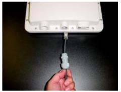
**Step 7:** Connect the RJ-45 to the female connecter located directly inside the enclosure, make sure the connection is locked in place before tightening the gland.
