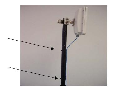
**Tip** For best results, secure this cable to the pole at least every 10 feet with tie-wraps.
