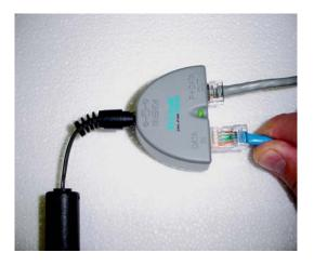
Caution Do not confuse the Ethernet input port with the Ethernet/Power output port. To avoid permanent hardware damage, make certain that you connect your backbone device to the Ethernet input port (not the Ethernet/Power output port).
