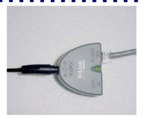
Step 5: Plug your Ethernet patch cable into the Ethernet input port (Data In) of the indoor unit and into the data port of your backbone device.
