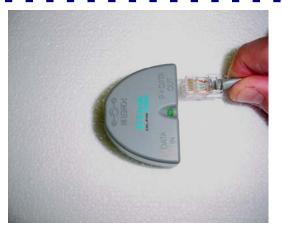
Caution Connecting any device other than the outdoor unit to the indoor unit may cause permanent hardware damage. Do not confuse the RJ-45 connector of the outdoor unit's with that of the Ethernet cable connected to your backbone device.
