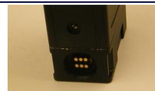
pack through a 5 pin POGO interface, 6 pins are used on the connector for ruggedness and alignment but the middle pin in the bottom row is unused. This port is potted with a sealant for waterproofing purposes and the SM has internal short-circuit protection but can be damaged if an external voltage is applied to the wrong pins. Please use only Raveon supplied assemblies for connection to this port.
